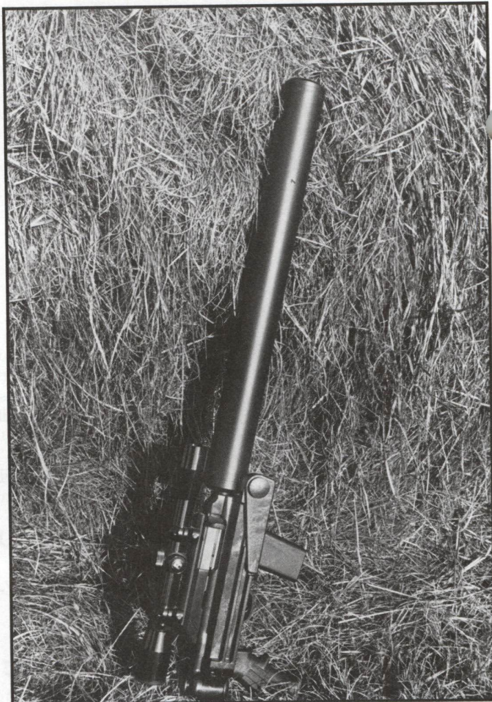
The Sound Technology suppressed Marlin Camp carbine produces only 1/1,000 the sound pressure level of an unsuppressed carbine. The folding stock reduces system weight by about a pound.
