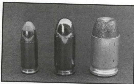
Mark White's .58 caliber subsonic pistol round (right) features a 550 grain bullet, while the .45 ACP (center) features a 230 grain bullet, and the Samson 9mm subsonic features a 158 grain bullet. White's case head is stamped "WHITE 58 AUTO".
