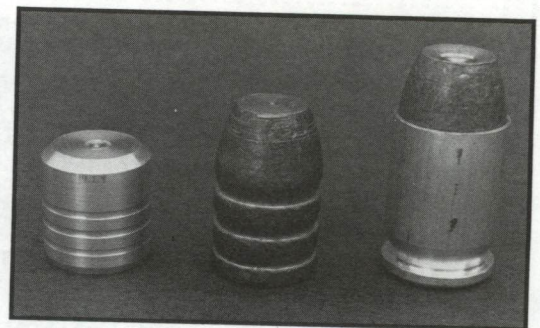
The "White .58 Auto" compared to a .58 caliber, 478 grain Minnie ball and an aluminum model of a .58 caliber semi-wadcutter (which would weigh 577 grains in lead) designed for White's pistol round.
