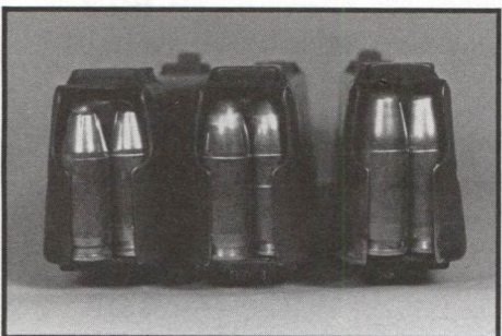
90, 115, 145 grain loads. Left to right: 90-grain loads caused "stove pipe" feeding jams. 115's fed without trouble.
